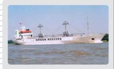
The vessel is fully gratings fitted and is built for a high flexibility for shipment of chilled/frozen cargo of both palletized and loose configuration.
